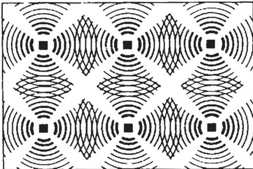
**Diagram IV-a: Spatial Infestations -** illustrates a solution for a widespread bird problem. The atmosphere is totally saturated by the use of multiple units. The sound waves overlap and cover the whole area.
