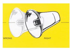
It is important to maximize the benefit of prevailing winds, to use these to enhance the distance that sound will naturally travel. If not considered, in positioning the loudspeakers, it could be that wind could reduce the distance that the dispersal sound will travel, blowing in the opposite direction to that which the loudspeakers are directed.
