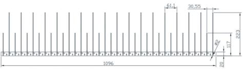
The Chimney pot spike is compatible with both large and smaller Pots. In the case of a smaller pot, the strap simply overlaps similar to a belt. Additional spikes can be removed where they have overlapped by choice.
