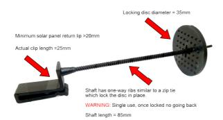
2.2.2 Roof covering: Kink the wire mesh as per installation instructions prior to offering up to solar panel frame. Then slide over sliding Solar Panel Bird Exclusion Clip and lock in position using non-return disc. No mechanical fixings will be necessary 2.2.3 Close internal and external corners using zip ties included in kit and
