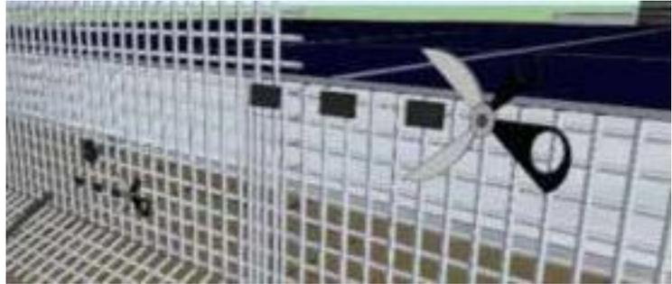
Outer Corner: Cut upwards from the bottom until the bend point. Bend the piece around the corner. Use the supplied stainless steel corner ties to joint the corners.
